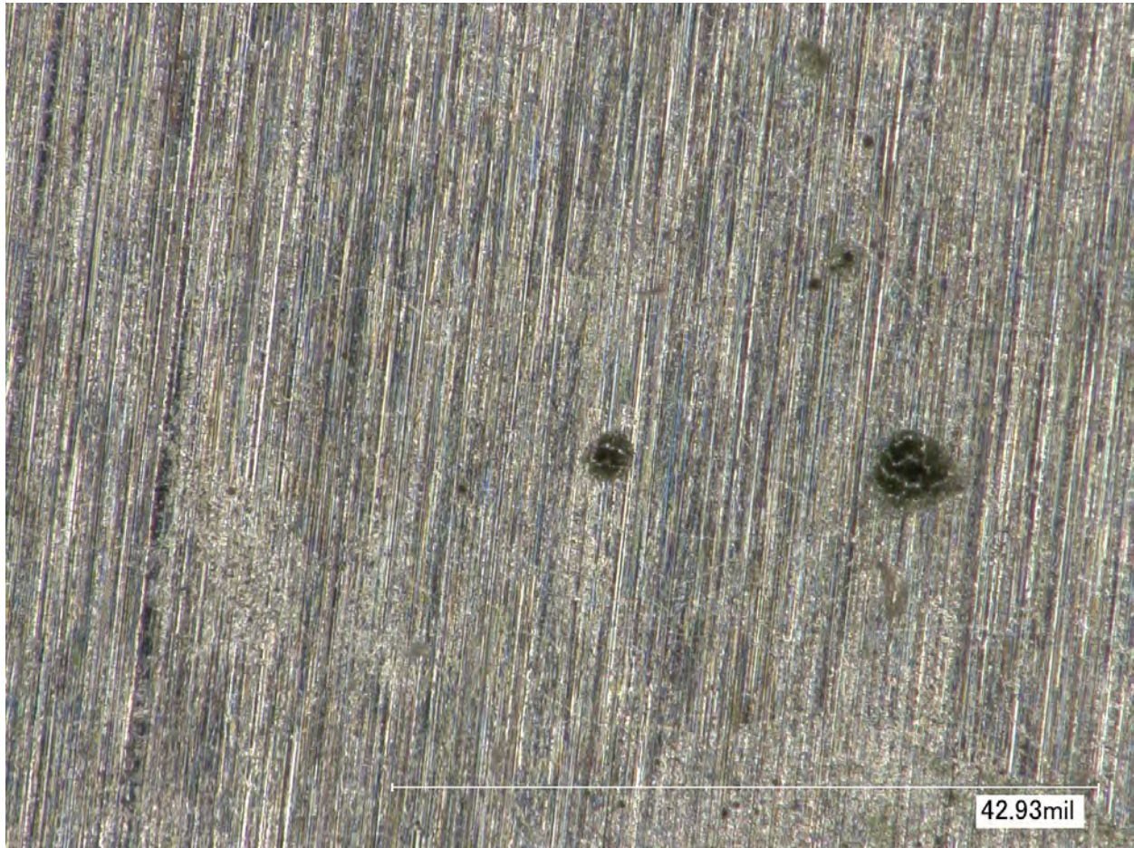
Figure 7 – MG1-3500* at 200x magnification exhibiting no growth and spore deposits
